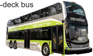
ADL Enviro500EV CHARGE Zero-emission, battery-electric, double-deck bus
