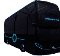
ADL H2.0 Next-generation hydrogen fuel-cell electric double-deck
