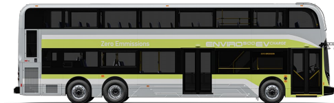
ADL Enviro500EV CHARGE Zero-emission, battery-electric, double-deck bus
